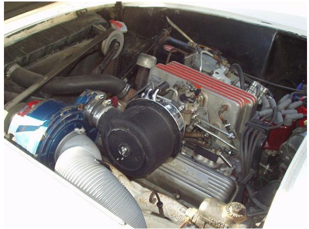
The 57 with fuel injection and a Paxton Supercharger
